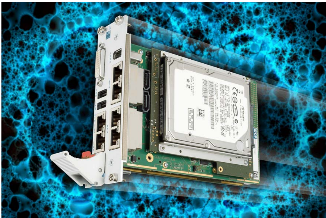
CCL-CAPELLA Side Board with CPU Carrier Card Assembly
