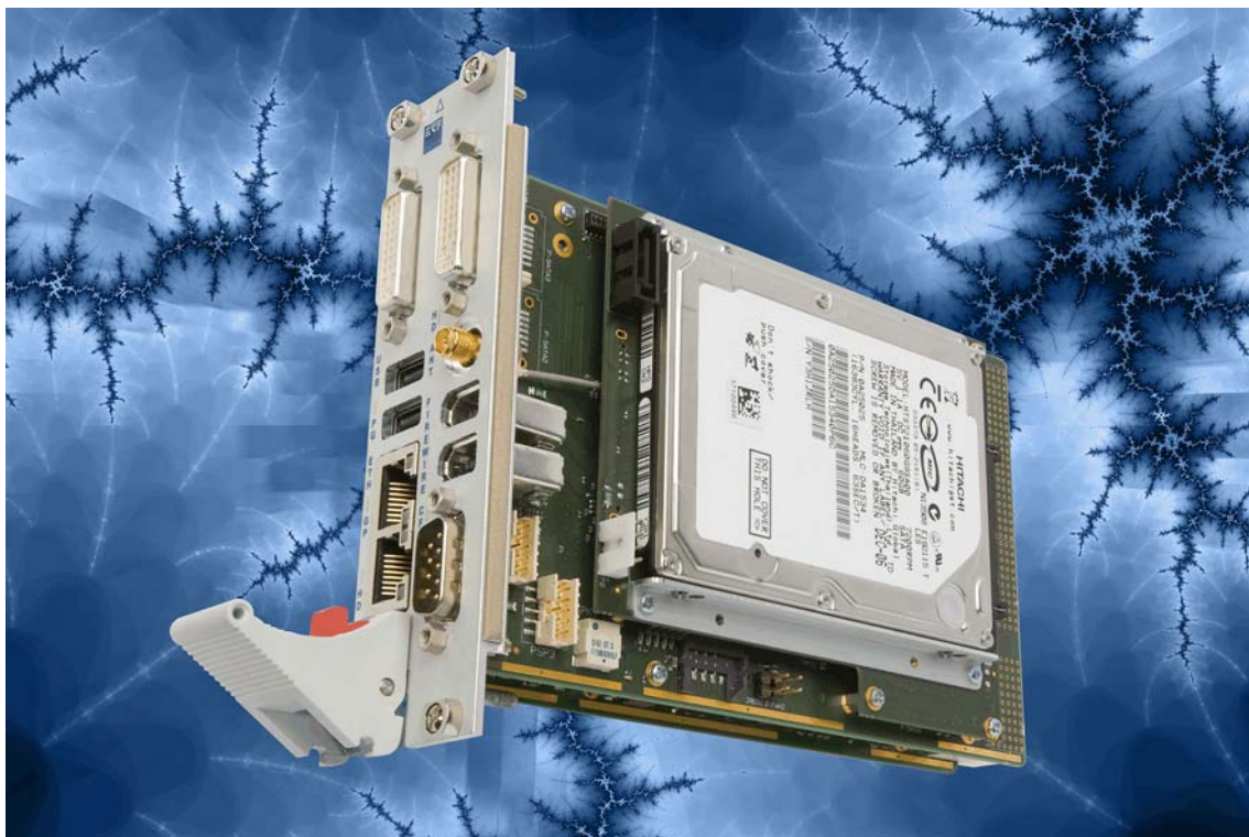
CCI-RAP Side Board on CPU Carrier Card Assembly
