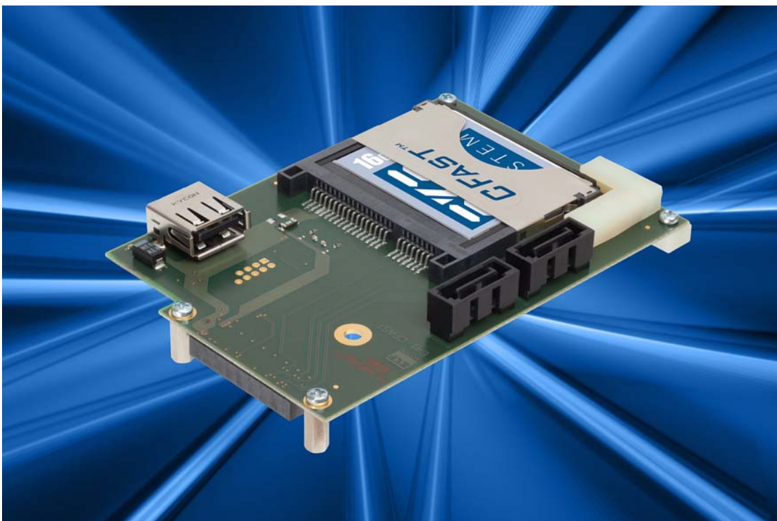
C41-CFAST SATA Based Storage Module
