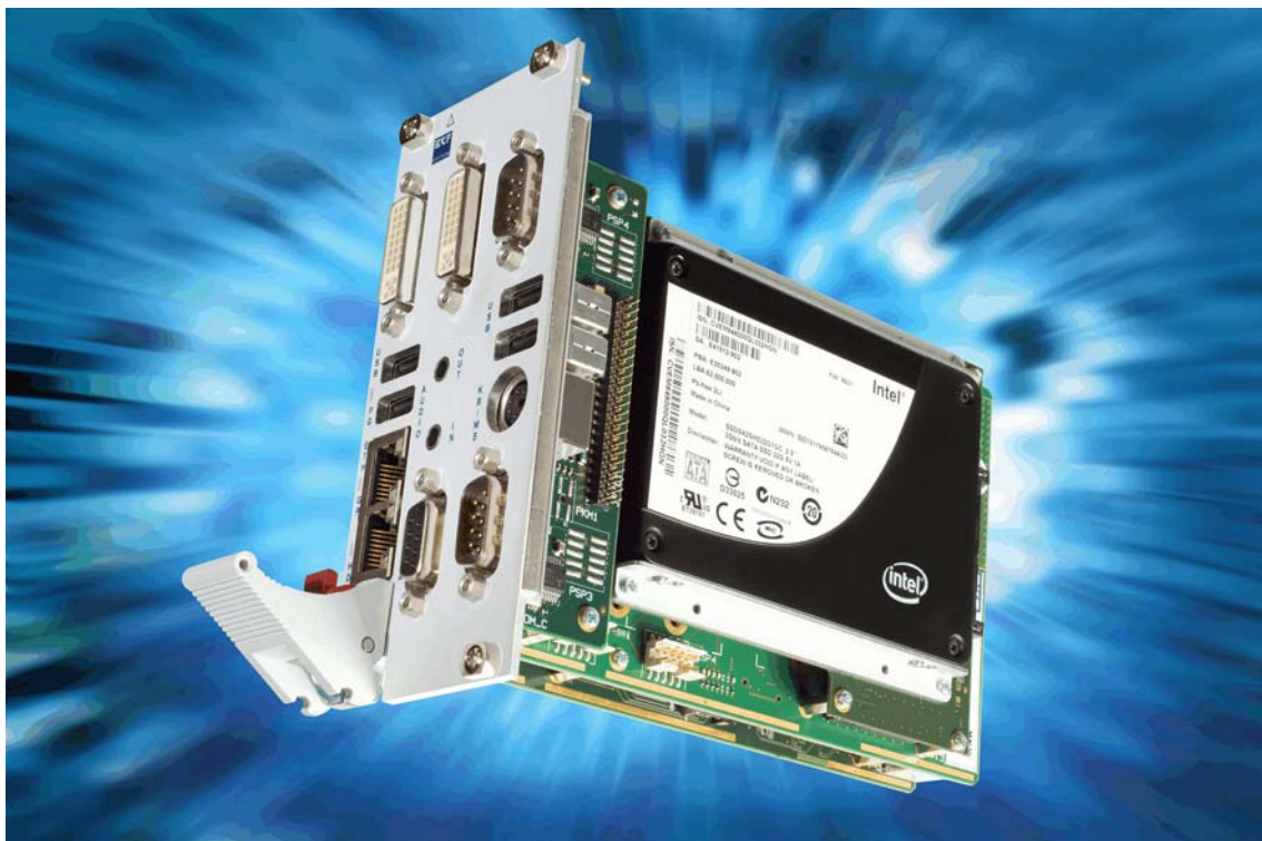
CCO-CONCERT Side Board & C20-SATA & C32-FIO with CPU Card Assembly
