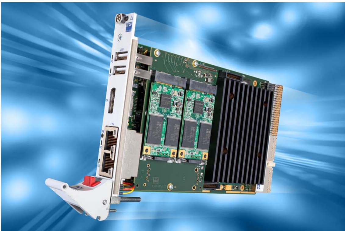
C47-MSATA SSD RAID Storage Module on CPU Carrier Card
