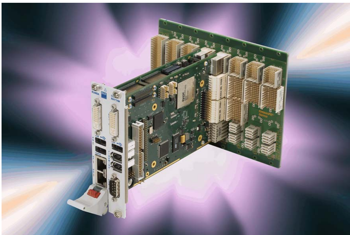
CPU Carrier Card w. CCJ-RHYTHM Side Board (Picture Similar)
