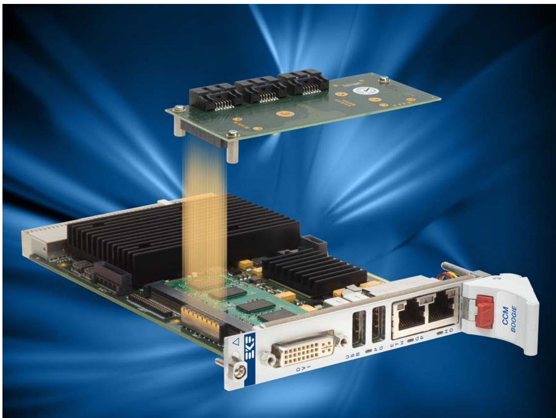
CCM-BOOGIE w. C43-SATA Internal Connectors Module
