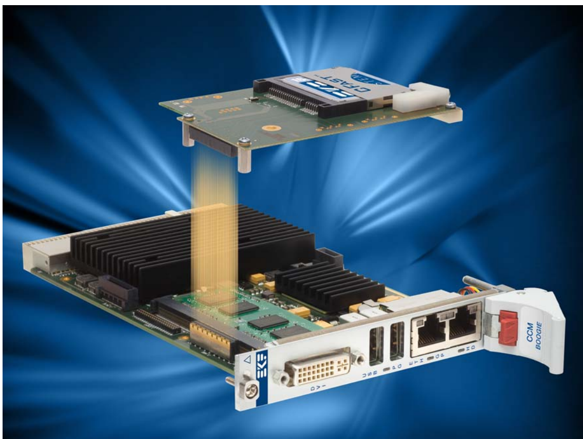
CCM-BOOGIE w. C41-CFAST Mezzanine Storage Module
