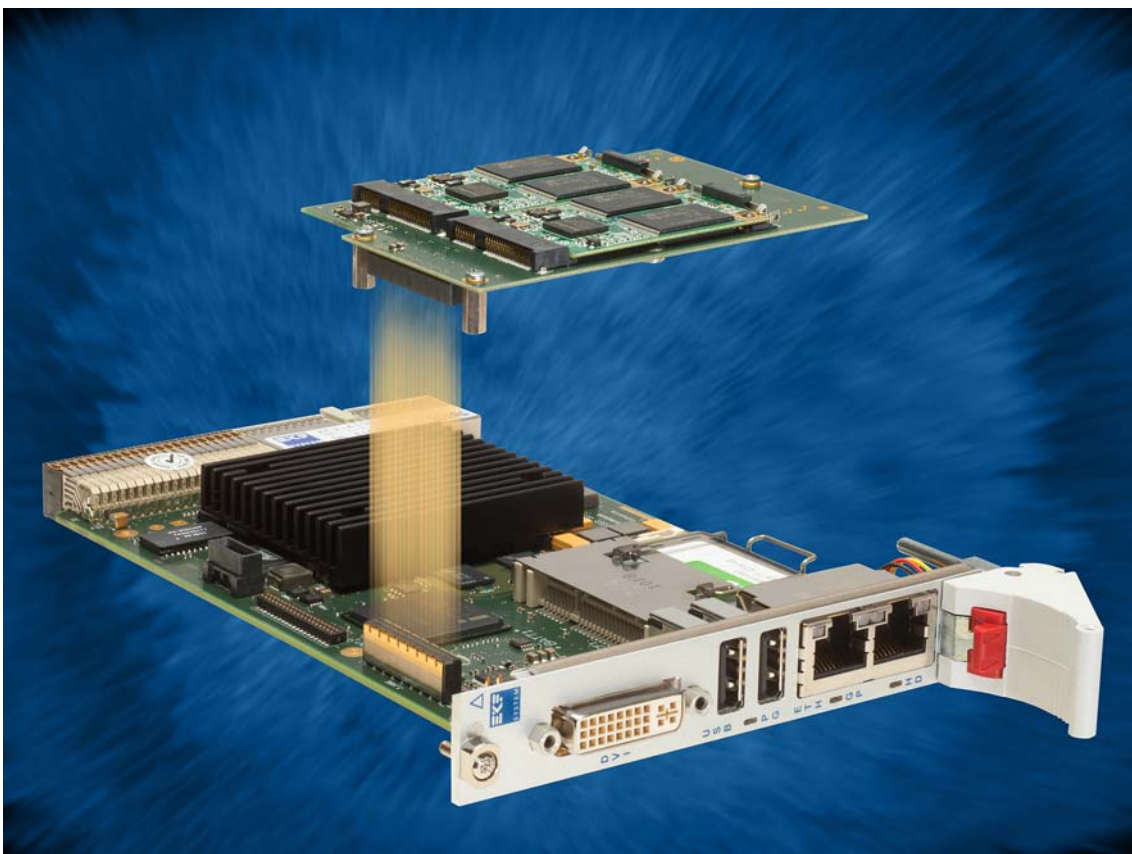
C47-MSATA over CPU Carrier Card
